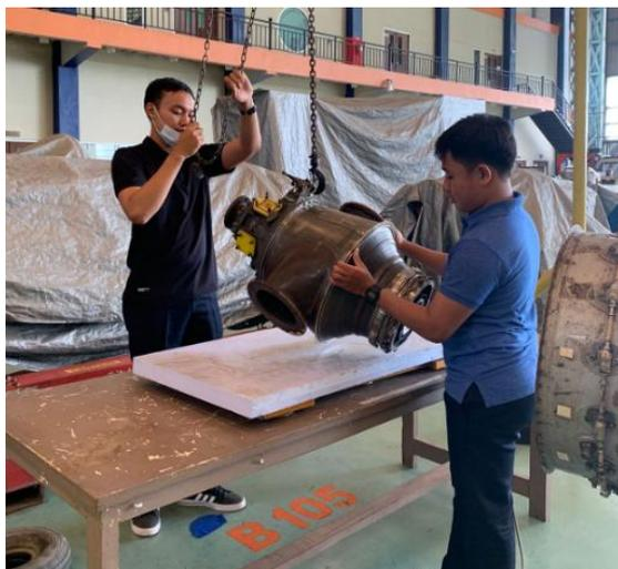
Gambar 4. Proses penimbangan *Engine* PT6-42.
